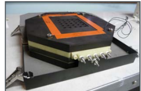
Twenty-five electrode fuel cell test fixture for combinatorial testing of fuel cell cathode performance
