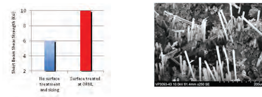
Figure 3. (a) Short beam shear test results of composites prepared from Zoltek Panex 35 fiber with vinyl ester resin (AOC 3045) before and after surface treatment at ORNL; (b) SEM image of fractured surfaces of non-surface-treated and unsized fibers with vinyl ester composites.
