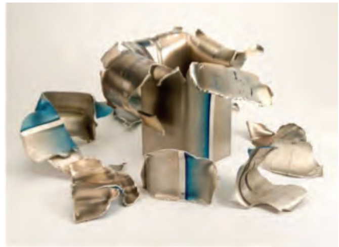
Figure 1. Mg extrusion exhibiting low ductility failure.
