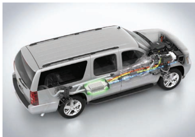
FIGURE 1. A Chevy Suburban with an Exhaust TE Generator
