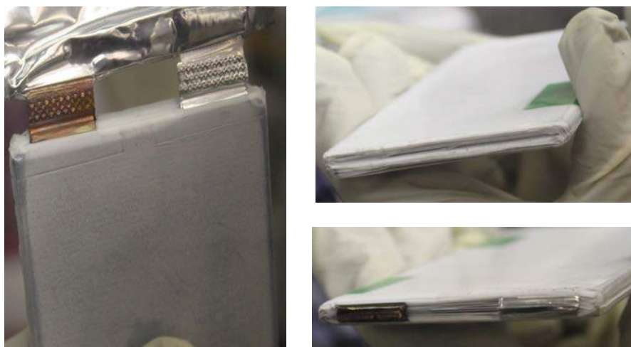
Figure ES- 1. Images of an 11 Ah capacity pouch cell undergoing teardown and failure analysis
