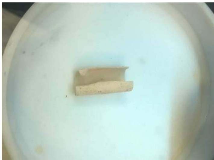
Figure II-486. Photograph of the flexible hybrid composite polymer electrolyte.
