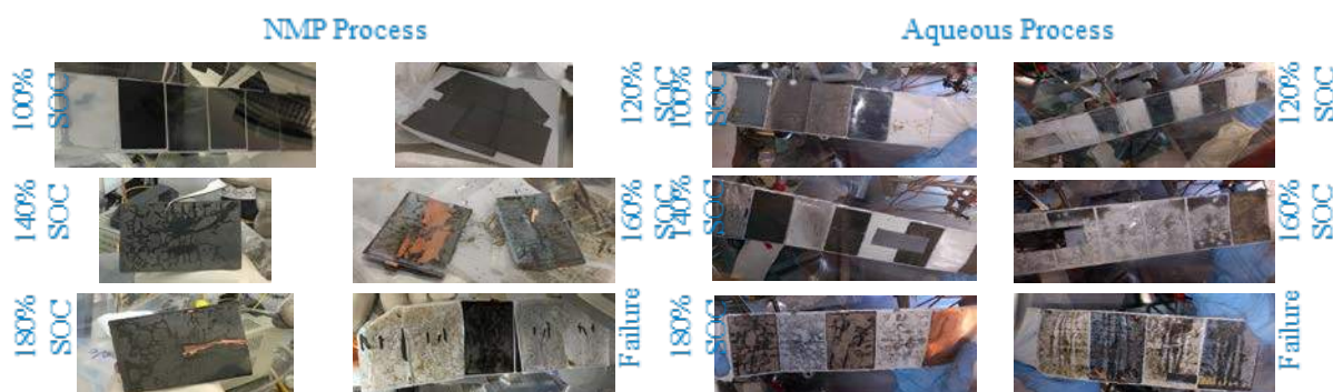
Figure II-440. Images of the anodes from the overcharged cells. The rectangular-shaped voids in some of the images are from sampling for microscopy.
