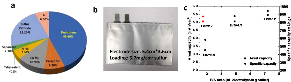
Figure II-563. (a) Component weight distribution of Li-S battery with energy density of 300 Wh kg -1 , (b) photo of single-layer pouch cell used in present study (Electrode working area 19.4 cm 2 and sulfur mass loading 5.7 mg cm -2 ), and (c) dependence of first-discharge areal capacity and specific capacity on electrolyte/sulfur ratio (black symbol - pouch cell using pristine separator; red symbol - pouch cell using modified separator).
