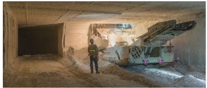
A continuous miner completes the initial rough cut of Panel 8, creating additional space for TRU waste disposal.
