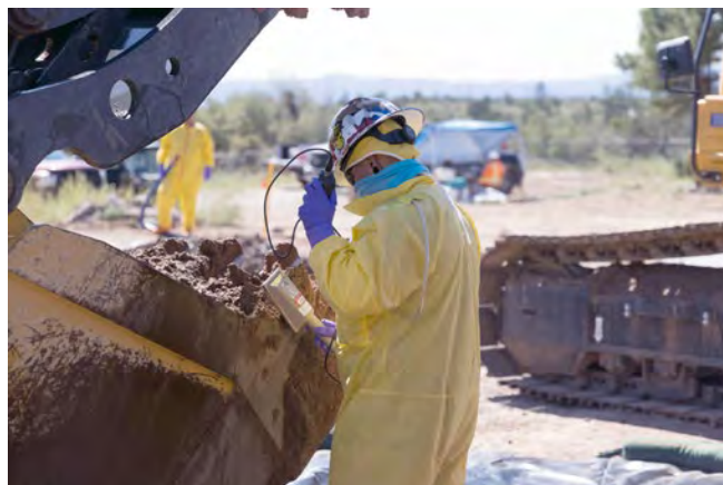
A crew worker screens debris mixed with soil for radiological activity.
