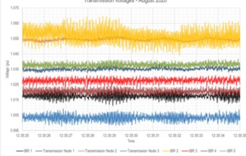
Fig. 15. AEMO 19-Hz oscillations - West Murray area.
