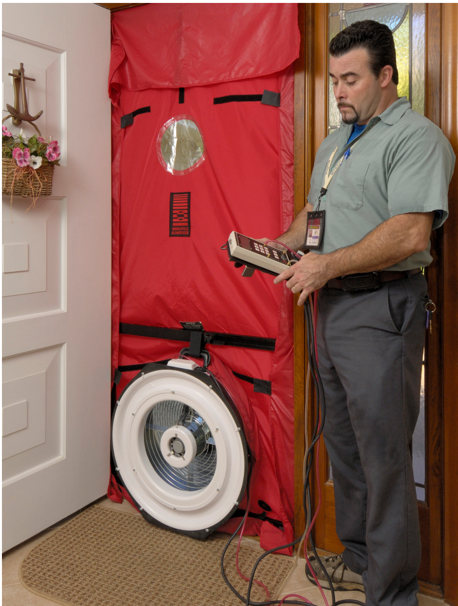
A blower door test helps evaluate a home's air tightness and is an important part of the initial assessment.
