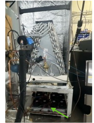
Integration of refrigerant-to-air TE HP
