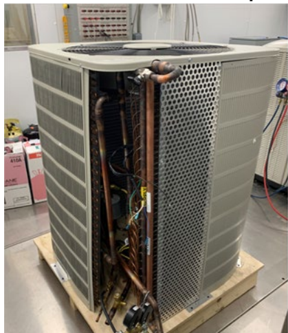
Outdoor 5 mm tube coil installed on 4.5 ton chasis
