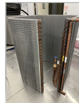
5-mm tube cross-counterflow outdoor coil
