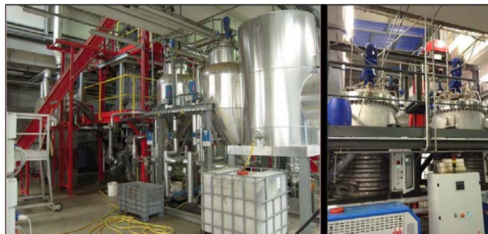
Pretreatment and Enzymatic Hydrolysis sections in the BioChemtex PROESA™ pilot plant
